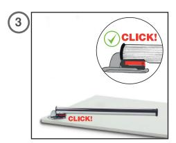
For correct use, open the leg until the safety lock snaps completely.
