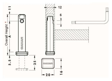
\*Overall Height O/A = (11mm + "A" + 5.5mm)"A" Height is from top of the foot to center of hole
